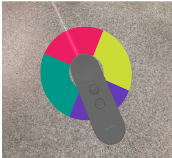
Figure 12: Addition of Swipe Menu to Daydream Controller in VR.
